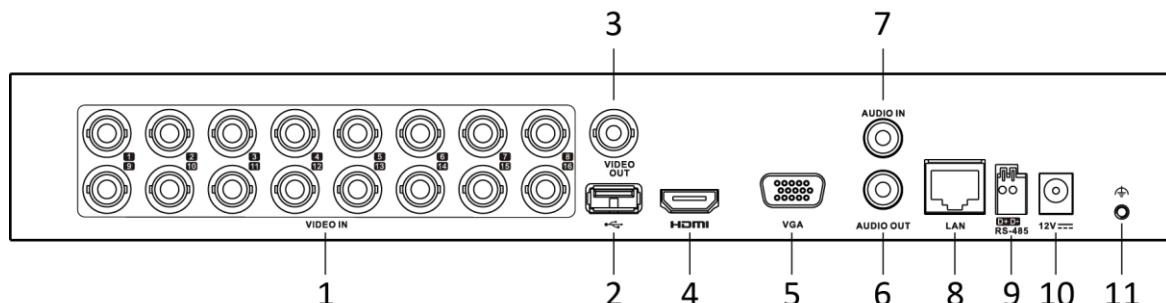
\*: The rear panel of iDS-7204HQHI-M1/S provides 4 video input interfaces. The rear panel of iDS-7208HQHI-M1/S provides 8 video input interfaces.
